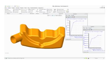
Creo BMX ensures your design meets its requirements. Here, we can ensure the designed tank will be able to hold the desired volume of fuel.
